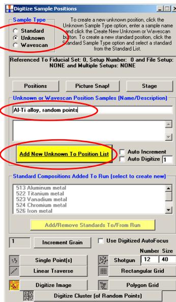
3. Then click on the 'Stage' button to bring up the 'Stage Map' window to navigate to the sample coordinates. Select the appropriate stage map image or drawing from the 'Holder Selection' drop down list.
