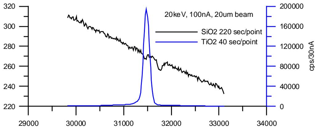
Fig 1. Wavelength dispersive scans on SiO<sub>2</sub> and TiO<sub>2</sub> at the position for Ti K $\alpha$  showing “holes” in the continuum both adjacent to and underneath the analytical peak.
