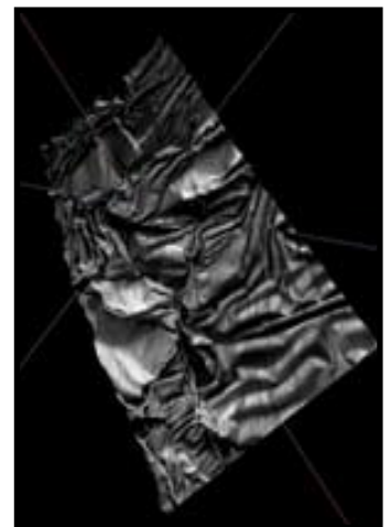
Reconstructed digital elevation model (DEM) of wrinkled glass surface at 500 x, using stereo imaging in the SEM
