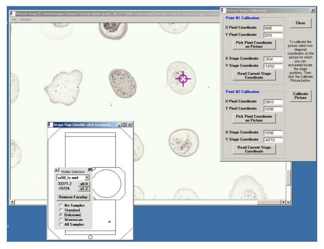
The current stage position location is shown as a target cursor on the calibrated picture and is updated continuously as the stage position is adjusted by the user. To move to any point on the image simply double click the image coordinate.
