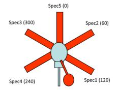
For JEOL instruments there are two types that will depend on the instrument model and/or regional differences. We document JEOL Type 1 as shown here:
