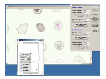
The current stage position location is shown as a target cursor on the calibrated picture and is updated continuously as the stage position is adjusted by the user. To move to any point on the image simply double click the image coordinate.
