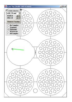
The standard, unknown and wavescan coordinates can be displayed on the stage bitmap. Also note the small "\_" button in the upper left which will minimize the Holder Selection frame as well as the small "@" just to the right which allows the user to easily calculate the exact stage bitmap calibration values which can then be edited into the PROBEWIN.INI file.
