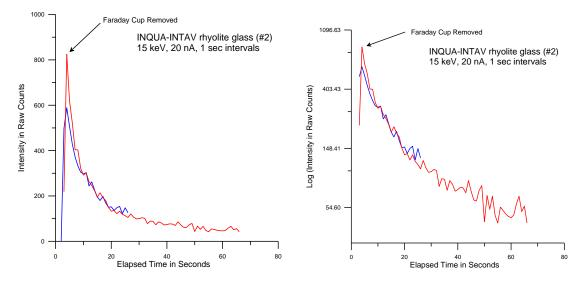
Note however, the slight curvature in the Lin-Log plot above (right hand side). This curvature in log space may indicate two separate exponential processes with different time constants overlapping in time. The "hyper-exponential" TDI correction described below is utilized to deal with this situation.
