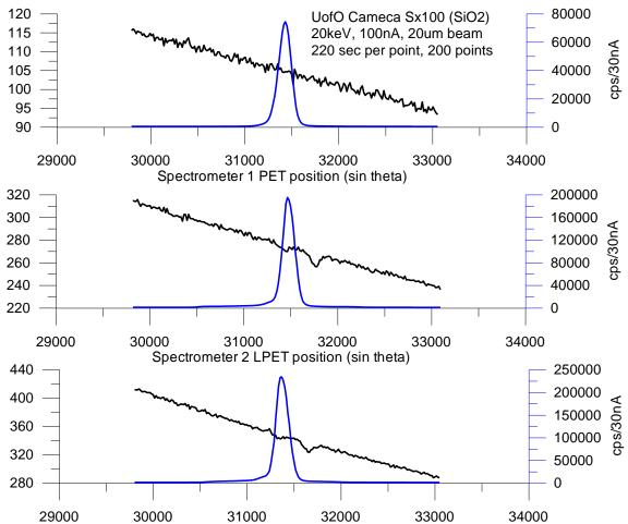
The following analysis is of a standard synthetic quartz with a Ti concentration of zero. The blank correction has been applied to itself to demonstrate the validity of the correction by calculating the intensity offset from the measured concentrations and calculating the resulting concentrations (which should be zero). Note the fact that the P/B values are very close to unity.
