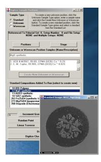
This can be used to check that you are on the correct standard or the image could be annotated to suggest places or grains to avoid during the standard digitization or acquisition process.
