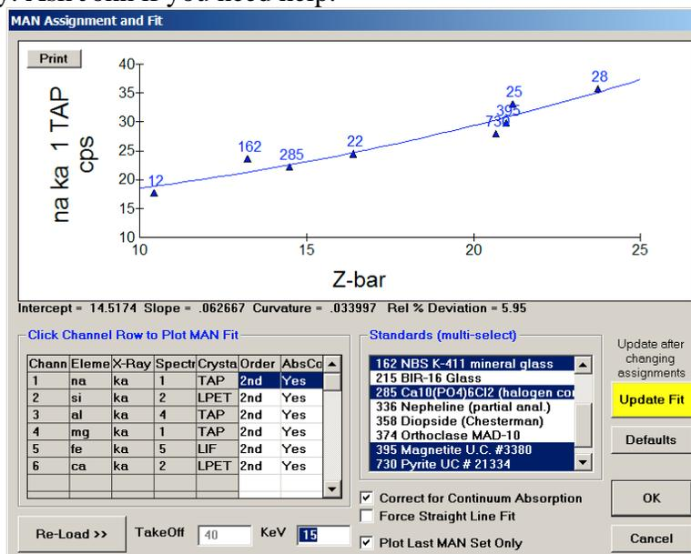
3. It is useful to run some standards that contain none of the elements you are analyzing for in order (and samples that are not used as the standard for a particular element!) to check that you are getting accurate measurements.
