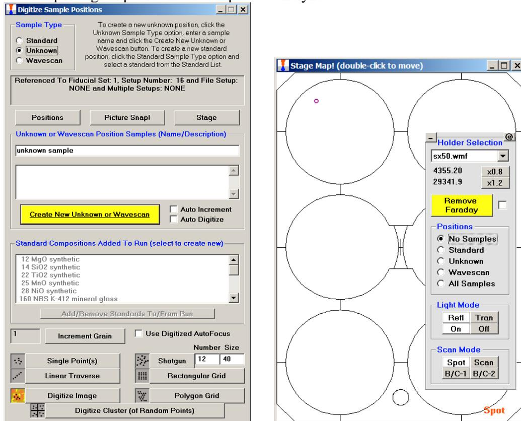
2. In the ‘Digitize Sample Positions’ window choose Unknowns and put a sample name in where you see -Unknown Sample- or a previous sample name you typed in and click Create a new Unknown or Wavescan then click on the Stage button to bring up the ‘Stage Map’ window.
